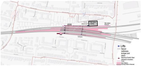
Providing a fast line up platform reduces the need for extra tracks and land—take north of Bromham Road and the need for a rebuild (or such an extensive rebuild) of Bromham Road bridge. It does this by enabling East Midlands Railway trains to stay on the fast line, so there is no danger of passenger delays on one route being transmitted to cause delays on another. This can be done most cheaply by
